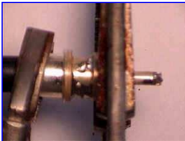
Soldered Center Conductor and Top Two Holes
