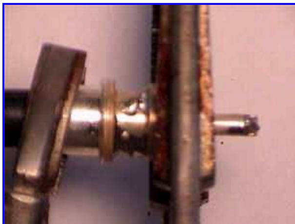
Soldered Center Conductor and Top Two Holes
